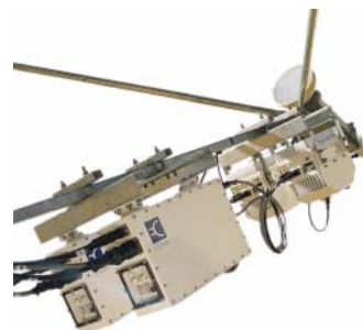
5700 transceivers antenna mounted in 1:1 configuration
